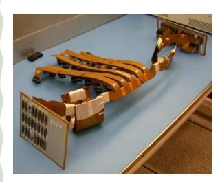
• Rigid/flex cabling. When available space and mass are a premium rigid/flex cabling may provide the answer. The two cables shown to the right provided all the interconnect requirements on the Mars Pathfinder rover. At 30 layers they were the highest layer count produced by our fabricator at the time, but through the use of tried and true design guidelines they achieved normal yields.
